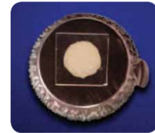
• After 300 cycles: Remains tacky with zero pump out
